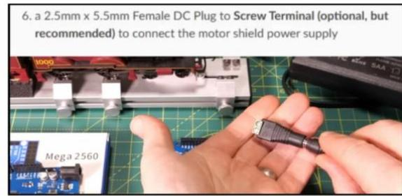
6. a 2.5mm x 5.5mm Female DC Plug to Screw Terminal (optional, but recommended) to connect the motor shield power supply
