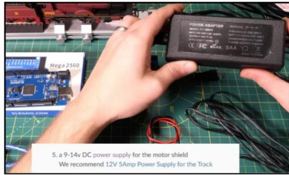
5. a 9-14v DC power supply for the motor shield
