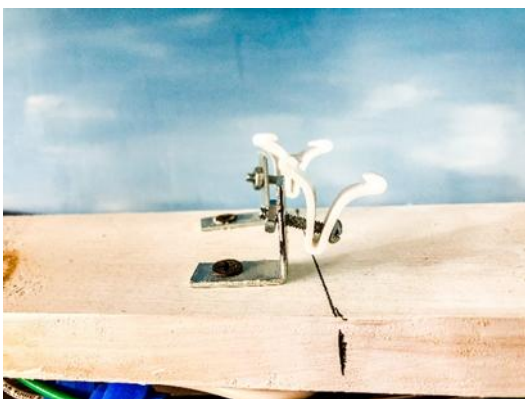
Photo 3 – Clips and corner brace attached to the 1 X 4. Note that I offset the metal brace so the clip is centered over the line.
