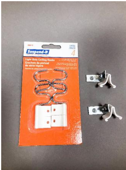
Photo 1 – Light-weight ceiling grid clips are the key. Attach them to 1" corner braces using 1" 6-32 machine screws.
