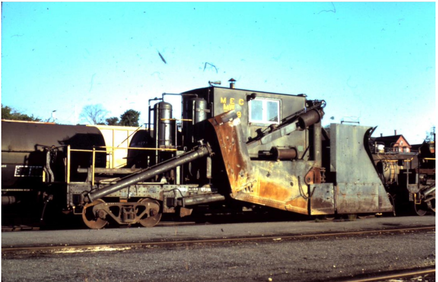
Maine Central Jordon Spreader , photo by Geoff Anthony
