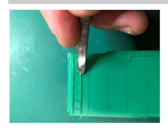
Fig. 1 Using a chisel to remove the plastic molded ladder
