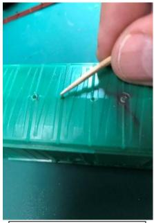
Fig. 3 Drill new holes for the Kadee running board and fill in the unused holes.
