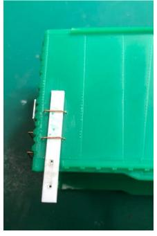
Fig. 7 Jig for uniform grab iron depth.
