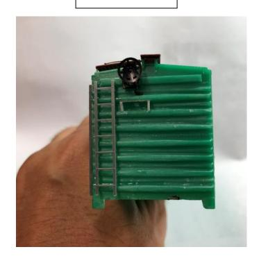
Fig. 8 B end with added ladder, brake housing and platform.
