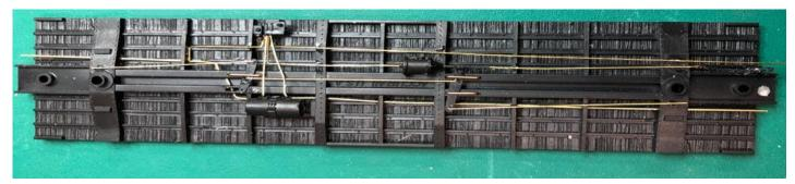
Fig. 4 Completed undercarriage AB brake parts with air lines.
