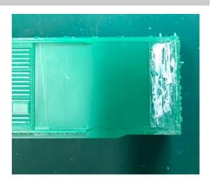
Fig. 2 Use putty to smooth over any gouges
