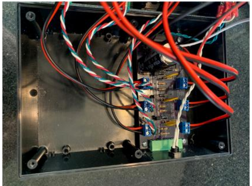
Figure 7 Power Supply Subassembly Installed in the lid
