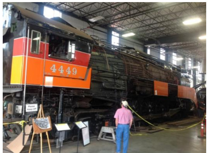
Tom Jones surveys the details of the stay bolts on SP 4449 undergoing overhaul at the Oregon Rail Heritage Center
