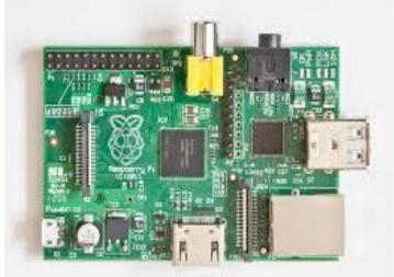
The Raspberry Pi is a low cost, **credit-card sized computer** that plugs into a computer monitor or other device.
