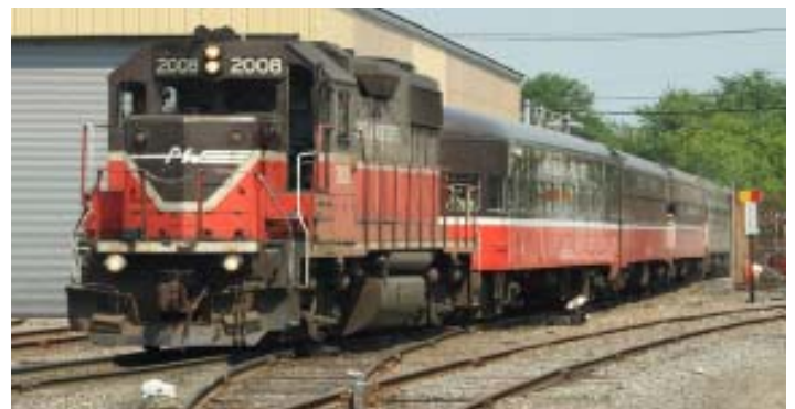
EMD GP38s, over 900 of them built by Electro-Motive Division of General Motors from 1966 to 1971. Some of are still active in New England. Many have been rebuilt, updated and kept in service by railroads, including Amtrak, N&W and P&W seen on this page. For model railroaders, Atlas has released Santa Fe and BNSF versions of the GP38 in conventional DC or in DC/DCC with QSI Sound. Prototype photos by Ron Palmquist
