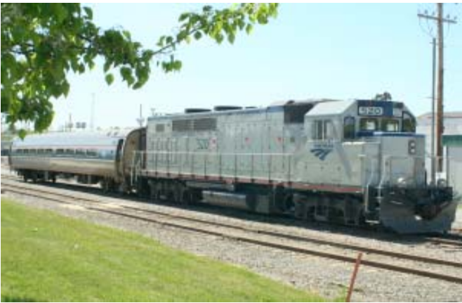
Amtrak 520, a GP38H-3 and a spare Amcoach, rest at the Portland Railroad/Bus depot awaiting service on the Downeaster passenger train to Boston. Usual power westbound is an Amtrak Genesis unit pushing, and an Amtrak exF40PH power unit (Cabbage) leading. Operating power trails on the Downeaster to avoid exhaust fumes and smoke from entering the covered platforms of North Station, the Boston terminus for the train.
