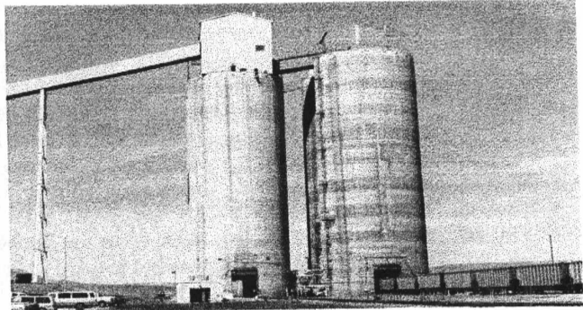
Flood-loading of WPEX gons at the Caballo Mine, Powder River, Wyo., August 11, 2002. - Stan Jordan photo
