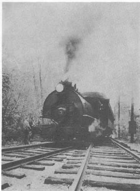
Squat ex-Hartford Electric Light Co. No.5 tries her drivers through the flangeways of the tie-plateless track whilst laying down a hail of cinders for the benefit of the open-end-platform coach riders and the two daisy-picking NER rail photographers.
