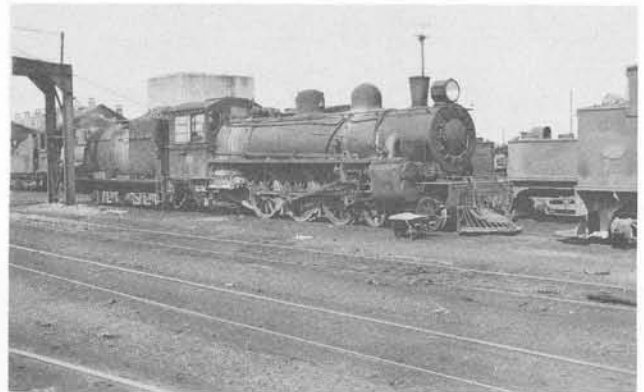
An A6 4-6-2 used in light passenger service in New Zealand. By Les Street
