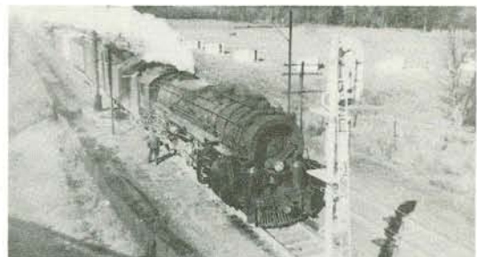
Boston and Maine 2-8-4 No. 4024 taking on water at Rockingham Junction, New Hampshire in April, 1946. Built by Lima, these were the work horses of the B.&M. Notice the Coffin heater on the front.
