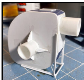
▲ FIGURE 4 - BLOWER WITH INLET AND OUTLET INSTALLED.
