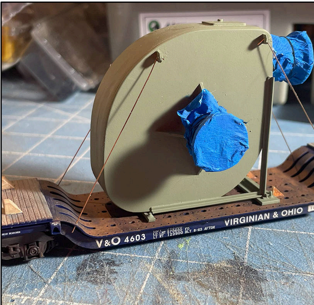
▲ FIGURE 11 - THE TIE-DOWNS IN PLACE. NOTE THAT THEY ARE ONLY GLUED TO THE LOAD, NOT THE FLAT CAR.
