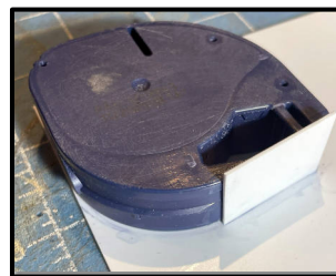
▲ FIGURE 2 - LAMINATING SHEET STYRENE TO THE CARTRIDGE.
