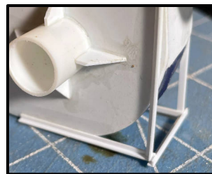
▲ FIGURE 3 - FRONT SUPPORT LEGS MADE OF 1/16" STYRENE ANGLE.
