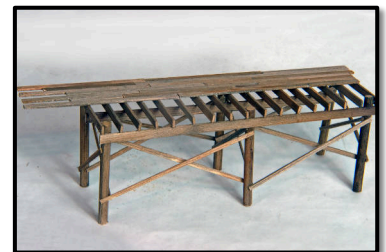
The lumber for under construction On30 dock were all cut with the Micro-Mark mini saw.
