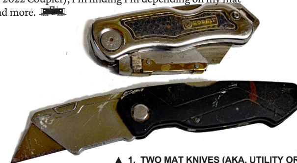
▲ 1. TWO MAT KNIVES (AKA. UTILITY OR BOX KNIVES) — ONE OPEN, THE OTHER FOLDED.
