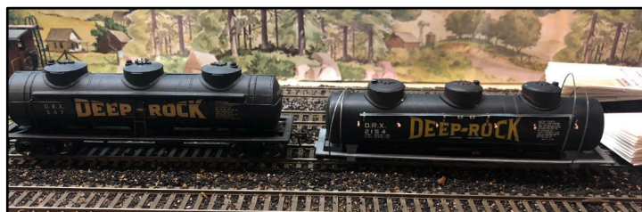
Figure 3: The Deep Rock tank partially assembled, next to its modern cousin. The tank bands needed to be glued at one end, and inserted into holes and bent on the other end. Two part epoxy glue was required as super glue didn't hold well enough.
