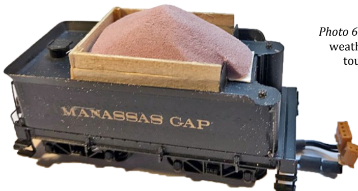
Photo 5: Shape the foam insulation to look like a coal load and hollow out the inside to fit around the capacitor.
