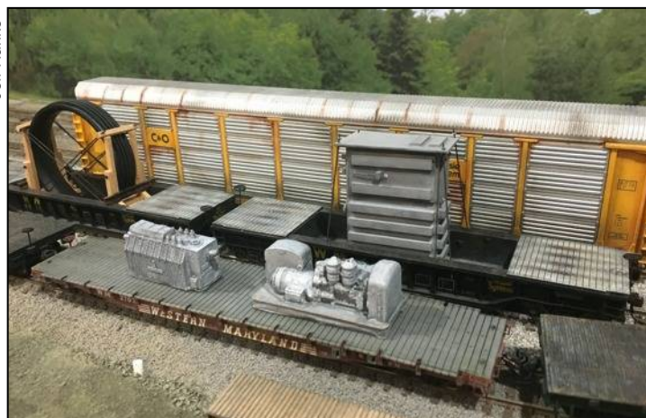
This collection of flat cars shows three of Chessie's four types. On the near track are three general purpose flats. The middle track holds two scratchbuilt well hole flat cars. These specialized cars are for hauling tall loads, as the floor of the car is low and close to the rails. Finally, in the background is an 89' multi-level flat car. These are tricky to use on home layouts with tight curves and may have to be excluded on some layouts.
