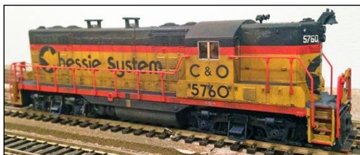
An Atlas GP7 was the starting point to adding Chessie appropriate details of spark arrestors, five-chime horn, and C&O-style nose mounted bell. There are also subtle details like evidence of the ACI card removed on the side sill, showing the old paint scheme underneath.
