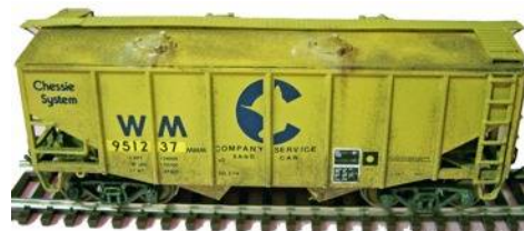
This MoW hopper shows off period details standard on my railroad. The COTS stencil and wheel inspection dot are Chessie Era features, as is evidence of post-1982 renumbering.
