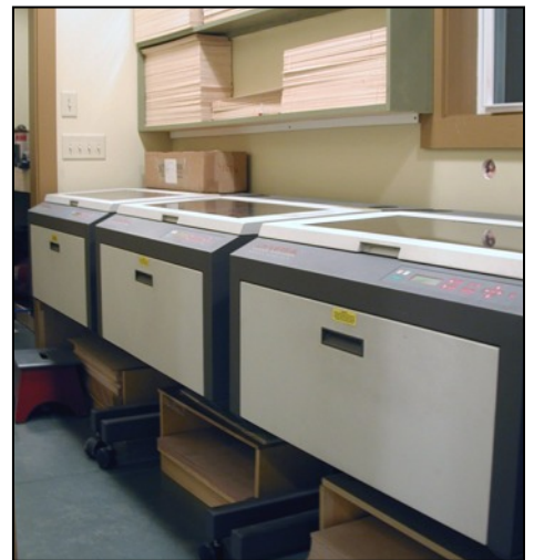
Laser cutters make accurate wood parts quickly and quietly with little waste and no sawdust.
