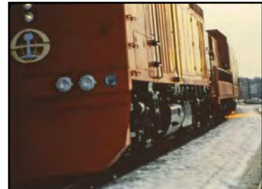
Because of the success of the RMS-1 train, Speno built the RMS-2. While the "power unit" is essentially an F40PH, the new cab featured a new nose design. The train also had more cars.
