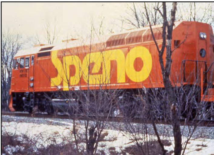
Side view of RMS-101 locomotive showing back, which was not changed from original F40PH. Below , sparks fly as the grinders reshape rail.
