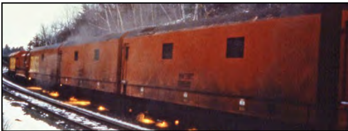
Side view of RMS-101 locomotive showing back, which was not changed from original F40PH. Below , sparks fly as the grinders reshape rail.
