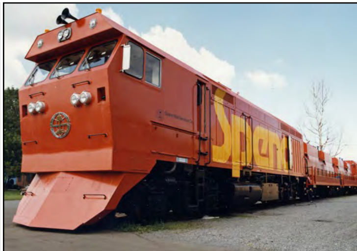
Because of the success of the RMS-1 train, Speno built the RMS-2. While the "power unit" is essentially an F40PH, the new cab featured a new nose design. The train also had more cars.
