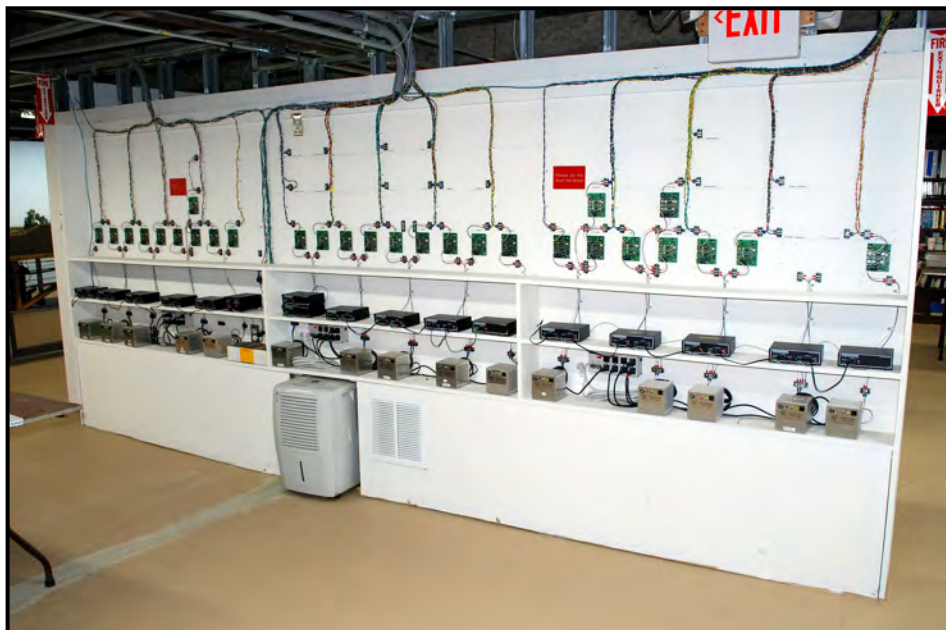
When completed, the DCC control system will have more than 25 boosters and many more individual circuit breaker protected track sections. This is the booster and breaker array. All connections to the layout pass over the aisle in a large conduit. A dehumidifier is located in the lower center of this wall section.
