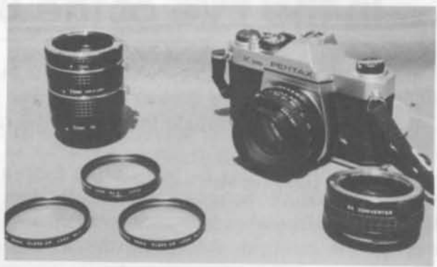
CLOSE-UP ACCESSORIES. Clockwise from the camera are: a 2x converter, a 3 piece set of close-up lenses and a set of extension tubes.
