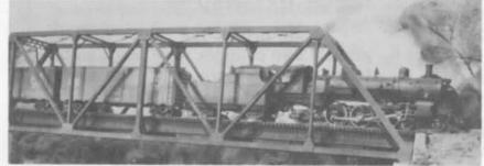
This S Gauge Pacific class J-3-b (Montreal Locomotive Works) was essentially scratch-built by Simon Parent of Val-Belair. The Sagami can motor uses a Dynatrol receiver. Building and rebuilding took 6 years.
