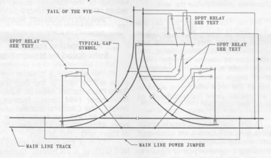
where operation naturally stops, allowing for reversal of the current. In a turning wye as shown in the illustration, the obvious choice is to let the direction sense of the tail control the polarity sense of the track.
