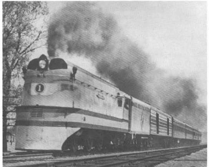
Back in the 1930's era streamlining was applied to many steam engines. Wind resistance was considered, but appearance of the clean outer shell was even more a factor
