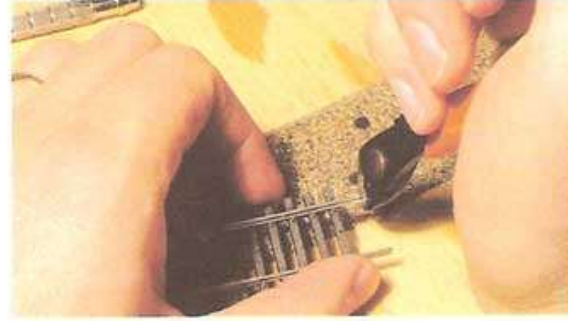
Fig. 9-17. Use rail nippers or a razor saw to cut the rail at the mark.
