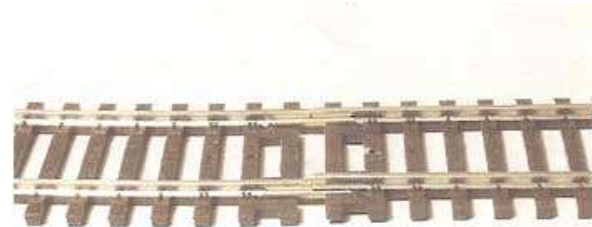
Rail joiner misaligned. Rail has slide over joiner.
