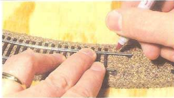
Fig. 9-16. Flex the end of the track into position, then mark the long rail at the point where it is even with the other rail end.
